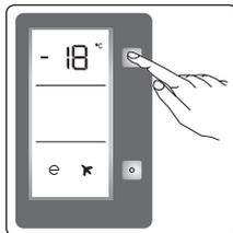
• The value for the freezer compartment will change to a lower temperature when you press this button while the indicator is flashing.
