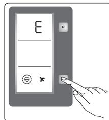
• If no button is pressed for 1 second, the mode will be set. The circle will blink 3 times and the buzzer will sound twice.
